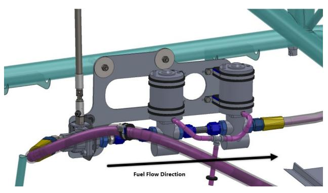
Figure 72-12 View of Fuel Pump System (Aircraft skin and frames not shown for clarity)
