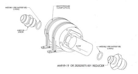
Figure 72-5 Exploded View of Main Fuel Pump
