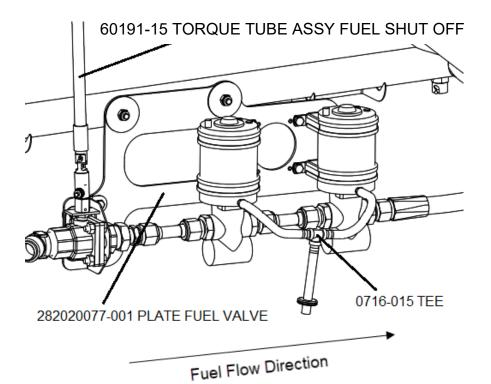
Figure 72-11 Fuel Shutoff Valve Torque Tube and Drain Tube Installation (Aircraft skin not shown for clarity)
