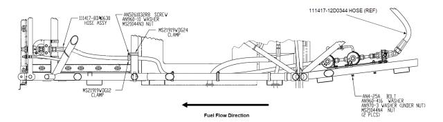
Figure 72-10 View of Fuel Pump & Filter System
