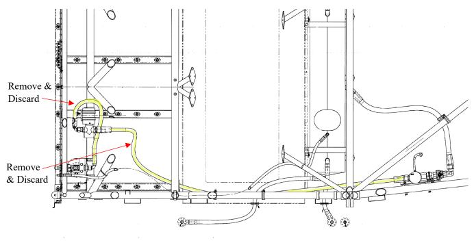
Figure 72-4 Fuel Pump & Filter System *Top View*
