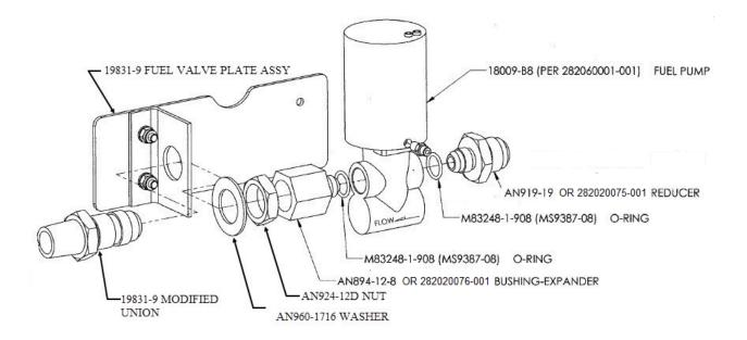
Figure 72-7 Exploded View of Emergency Fuel Pump
