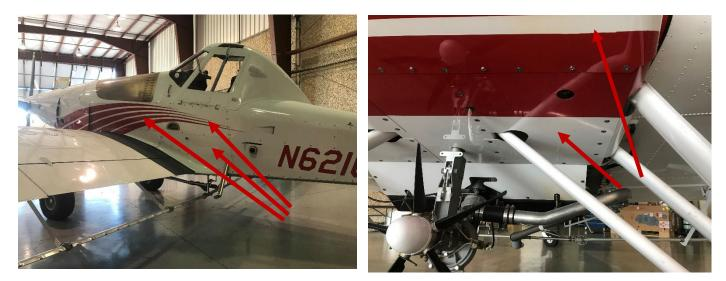
Figure 72-1 Emergency Fuel Pump Location
